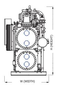
Side and front views of a Smardt V<sup>-</sup>Class Water-Cooled Chiller customized in a stacked configuration to fit a smaller footprint within a plant room. This example also illustrates a Pony Express configuration.
