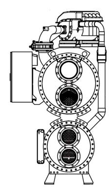
Side and front views of a Smardt T-Class water-cooled chiller customized in a stacked (narrow) configuration to fit a smaller footprint within a plant room
